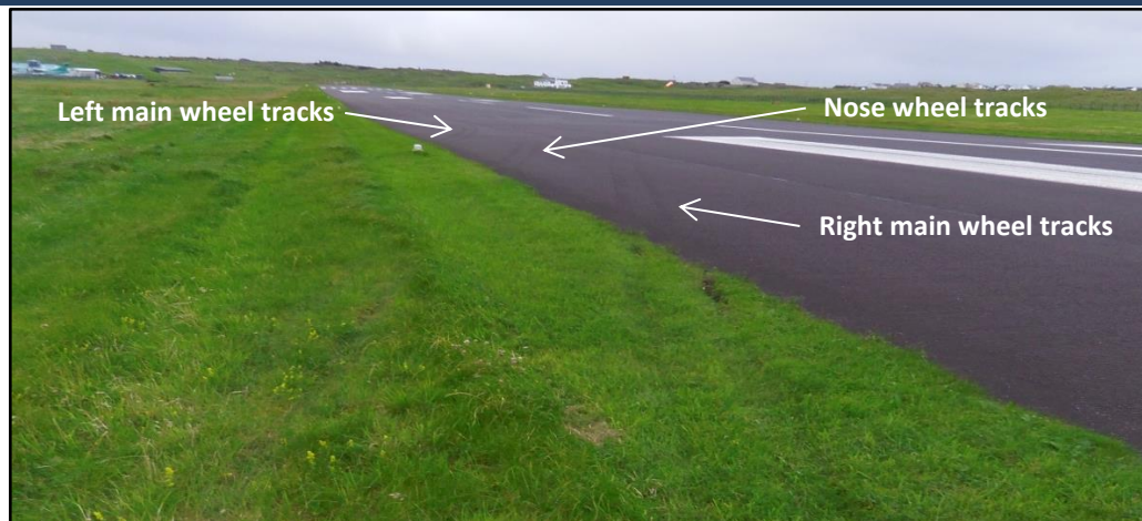
Photo No. 3: Tyre tracks indicating point of re-entry to the runway
